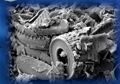
Scanning electron microscope image of Diafiltra® particles. Image size 20µm x 15µm.
